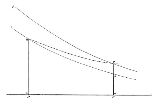
rature t and pressure p, and let the pressure be increased to p', the new volume a'b' of the gas will be less than  $ab\frac{p}{p'}$ . Let the gas be now heated at the pressure p' till its
